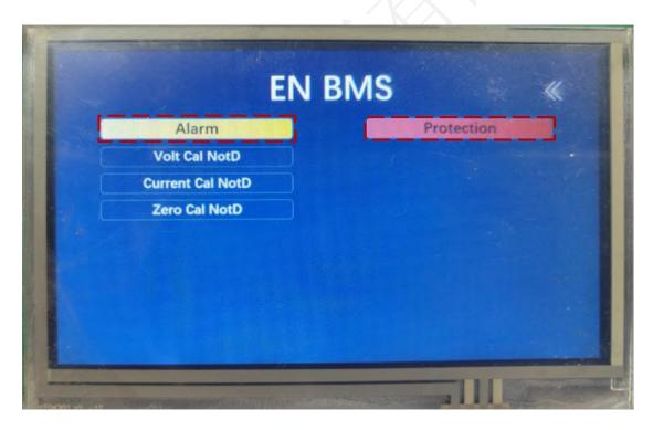
The above two pictures are in both Chinese and English states. Clicking on "Alarm" on the left or "Protection" on the right (yellow icon for alarm, red icon for protection) will display the specific alarm and protection items currently in use.
