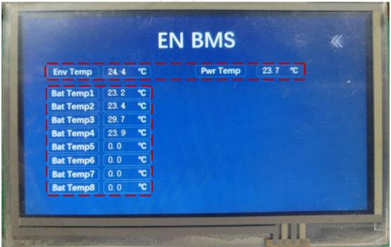
The above two pictures show the temperature details of each battery in both Chinese and English, including the current ambient temperature and power temperature.
